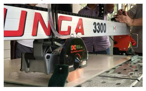
Keep the blade of the saw constantly wet in order to avoid that the heat caused by the friction produced by the saw that cuts the slab damages the glass.
