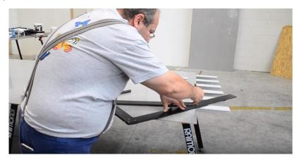
Once the cut has been made, it must be "opened" (meaning that the parts of the glass layer divided by the cut must be completely separated). This operation can be performed by hand or by using glass pliers.
